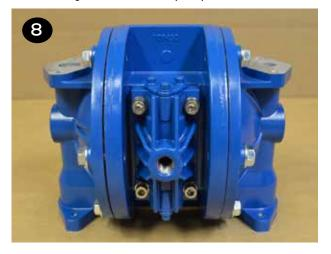
• Flip the pump upside down and drop the suction valve balls (item 15) into the liquid chamber (item 17) ball cages.
