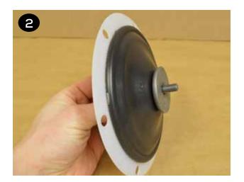
3 Apply a couple drops of a medium strength thread locker, such as Loctite® 246, to the outer plate bolt (item 19). Thread the shaft (item 27) onto the bolt until it is snug to the flat back side of the inner plate (item 22).
