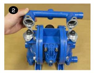
Repeat the above steps for the suction manifold (item12). The seat o-rings, valve seats and valve balls (items 13, 14, & 15) are located in the liquid chambers (item 18). Remove both liquid chambers by removing the (6) bolts (items 16) on each liquid chamber using a 13mm (or ½") wrench. Inspect and replace diaphragms if needed.
