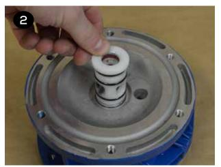
Inspect the shaft (item 27) for damage. It is common for shafts to become grooved during service. Grooving is normally caused by carbonized oil and/or abrasive foreign material getting trapped between the seal and the shaft. Over time, deep grooves can form in the shaft. When that occurs, it is recommended that the shaft be replaced.
