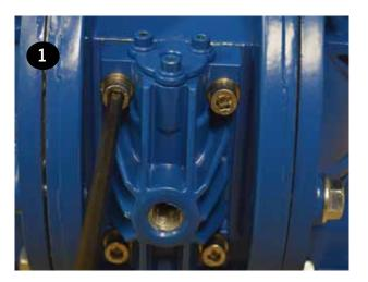
Pull the valve body and gasket (items 3 & 30) off the front of the center section (item 28) and the muffler plate gasket, muffler plate and muffler (items 29, 31 & 33) off the back.
