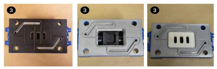
Insert the (4) cap screws & washers (items 1 & 2) through the valve body and gasket (items 3 & 30) and place onto the center section (item 28). Ensure the slide valve and valve plate (items 9 & 10) are in place and the valve sits flat on the center section.
