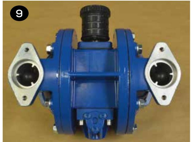
**10** install (1) of the valve seat o-rings (item 13) into the liquid chamber (item 17) followed by the valve seat (item 14) and then another valve seat o-ring (item 13). The o-ring will fit into the groove created by the valve seat and liquid chamber.
