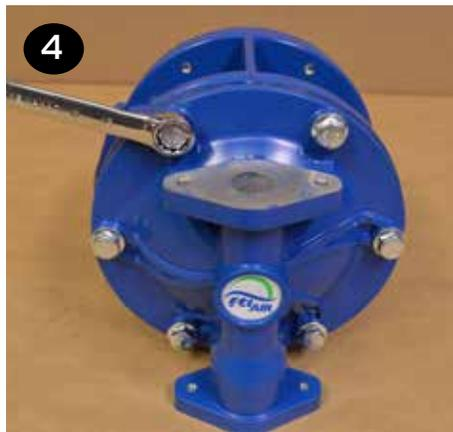
**5** To remove the diaphragms (items 20/ 21), begin by loosening the (2) outer plates (item 18) using 2-20mm wrenches. Use 6-sided sockets or wrenches to prevent damage to the hex portion of the outer plate.
