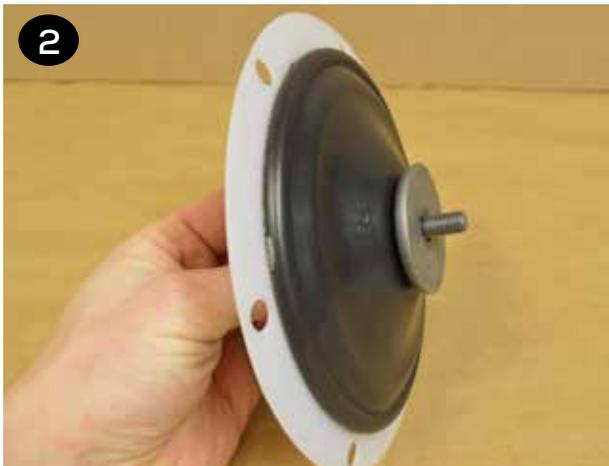
**3** Apply a couple drops of a medium strength thread locker, such as Loctite® 246, to the outer plate bolt (item 19). Thread the shaft (item 27) onto the bolt until it is snug to the flat back side of the inner plate (item 22).
