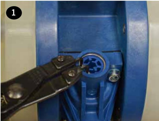
**1 Aluminum Air Valve** - To replace the valve cap o-rings (item 5), remove the (3) button head cap screws (item 7) using a 3mm hex wrench.
