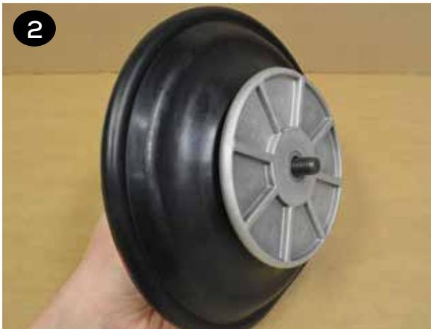
**3** Apply a couple drops of a medium strength thread locker, such as Loctite® 246, to the cast/threaded outer plate bolt (item 19). Thread the shaft (item 27) onto the bolt until it is snug to the flat back side of the inner plate (item 22).
