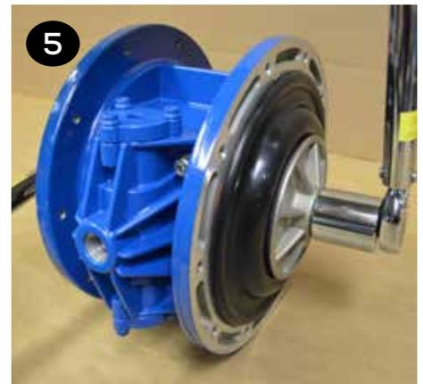
**6** Remove the outer plate, diaphragm(s), and inner plate (items 18, 20/21 & 22) from the side that is loosened. Pull or push the shaft (item 27) and remaining plates and diaphragms out of the center section. If pulling, it may be easier to grip the diaphragm if it is inverted.
