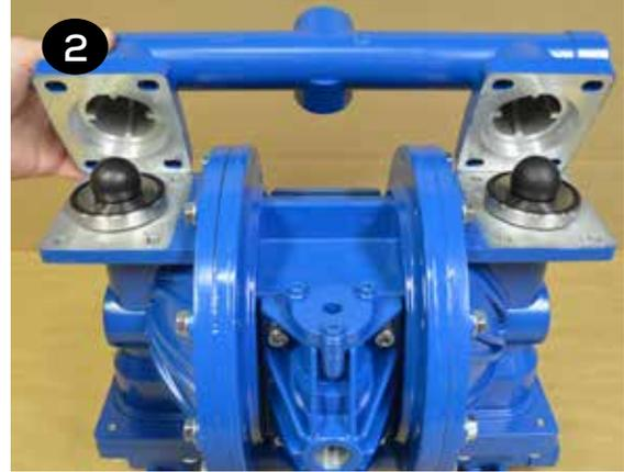
**3** Repeat the above steps for the suction manifold (item 12). The seat o-rings, valve seats and valve balls (items 13, 14, & 15) are located in the liquid chambers (item 17).
