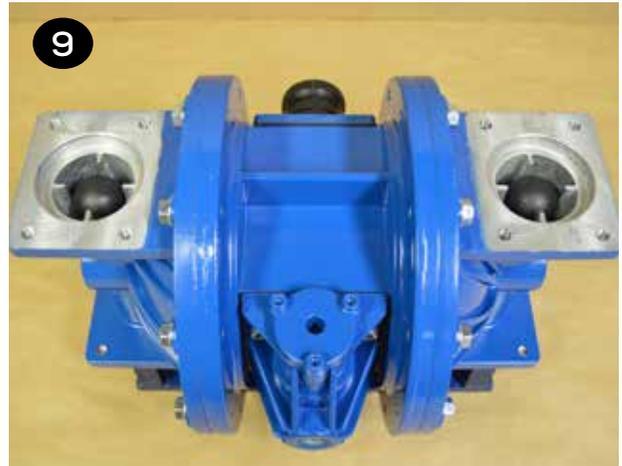
**10** Install the valve seat o-rings (item 13) into both sides of the valve seat (item 14). Install the valve seats into the liquid chambers. Valve seats are symmetrical.
