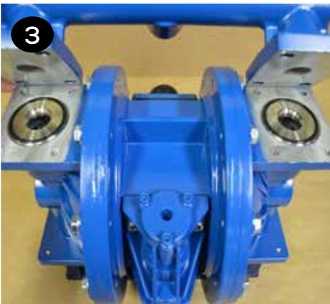
**4** Remove both liquid chambers (item 17) by removing the (10) bolts (item 16) on each liquid chamber using a 13mm (or ½") wrench. Inspect and replace diaphragms if needed.
