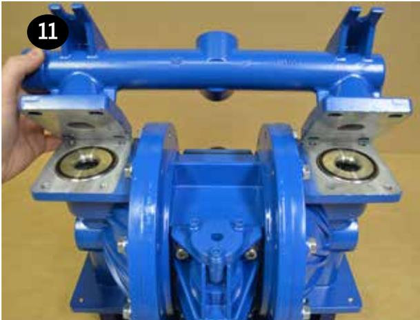
**12** Stand the pump upright onto the suction manifold feet (item 12). Install the valve seat o-rings (item 13) into both sides of the valve seats (item 14). Place the valve seats on top of the liquid chambers (item 17), followed by the valve balls (item 15) on top of the valve seats. The valve seats are symmetrical. Place the manifold atop the pump, over the components that are stacked on top of the liquid chambers. Install, tighten and torque the manifold bolts (item 11).
