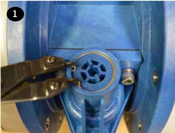
**1 Aluminum Air Valve** - To replace the valve cap o-rings (item 5), remove the (3) button head cap screws (item 7) using a 5mm hex wrench.
