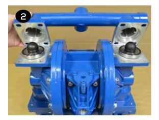
Repeat the above steps for the suction manifold (item12). The seat o-rings, valve seats and valve balls (items 13, 14, & 15) are located in the liquid chambers (item 17). Remove both liquid chambers (item 17) by removing the (10) bolts (item 16) on each liquid chamber using a 13mm (or ½") wrench. Inspect and replace diaphragms if needed.
