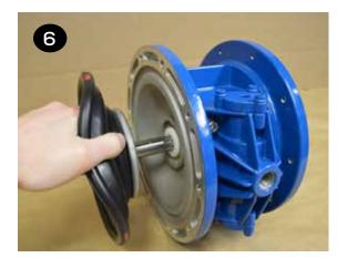
To remove the remaining diaphragm(s) (items 20/21) and plates (items 18 & 22) from the shaft (item 27), place the shaft in a vise fitted with soft jaws. Using a 6-sided 30mm wrench, remove the remaining diaphragm(s) and plates. Soft jaws are required to prevent damaging the shaft. A damaged shaft will result in accelerated o-ring wear. Jaws can be fitted with wood, plastic, rubber, or other soft material to prevent shaft damage.
