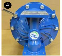
• To remove the diaphragms (items 20/21), begin by loosening the (2) outer plates (item 18) using 2-30mm wrenches. Use 6-sided sockets or wrenches to prevent damage to the hex portion of the outer plate.
