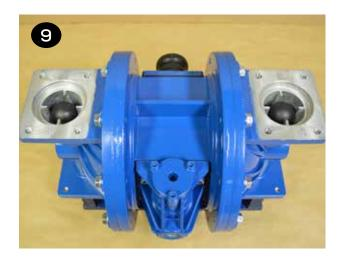
Install the valve seat o-rings (item 13) into both sides of the valve seat (item 14). Install the valve seats into the liquid chambers. Valve seats are symmetrical.
