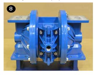
Flip the pump upside down and drop the suction valve balls (item 15) into the liquid chamber (item 18) ball cages.
