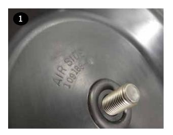
Place the inner plate (item 22) over the molded in bolt. Ensure the round recess in the plate faces the diaphragm (item 21).
