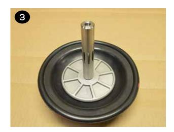
4 The shaft (item 27) and shaft o-rings (item 26) should retain the lubricant that was factory applied. If they appear dry, apply a light coat of lithium thickened grease. Avoid over lubrication as it can cause decreased performance of the air distribution system.
