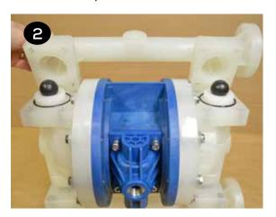
Repeat the above steps for the suction manifold (item12). The seat o-rings, valve seats and valve balls (items 13, 14, 15 & 16) are located in the liquid chambers (item 18).
