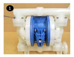
The discharge seat o-rings, valve seats, and valve balls (items 13, 14, 15 &16) can now be accessed and replaced if needed.
