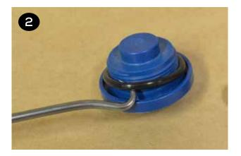
Aluminum Air Valve - Remove and replace o-ring (item 5). Install cap (item 6), tighten, and torque the valve cap screws (item 7). Repeat for the remaining cap.
