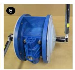
Remove the outer plate, diaphragm(s), and inner plate (items 19, 20/21 & 22) from the side that is loosened. Pull or push the shaft (item 27) and remaining plates and diaphragms out of the center section. If pulling, it may be easier to grip the diaphragm if it is inverted.
