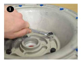
Remove and set aside the air valve (item 3) using a 6mm hex wrench (see Valve and Muffler Gasket Replacement section for more details). The shaft bushings can be removed by placing a large socket between the two bushings. Place and extension into the socket from one side of the center section. Tap with a rubber mallet to remove the bushing. Repeat for the remaining bushing.
