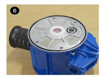
Install air chambers (item 26) by placing one side on top of the center section (item 35). Ensure the air path hole of the center section lines up with the through hole in the air chamber.
