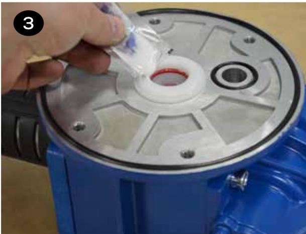
**4** Insert both bushings into the center section. Ensure the bushing is fully installed and the large rib on the outside of the bushing is flat against the center section.
