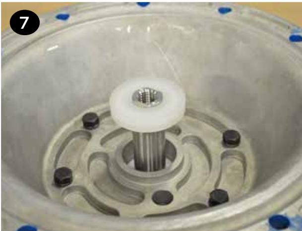
**8** It may be easier to thread the bolt into the shaft if the diaphragm(s) is inverted on one or both sides. This can be done by hand.
