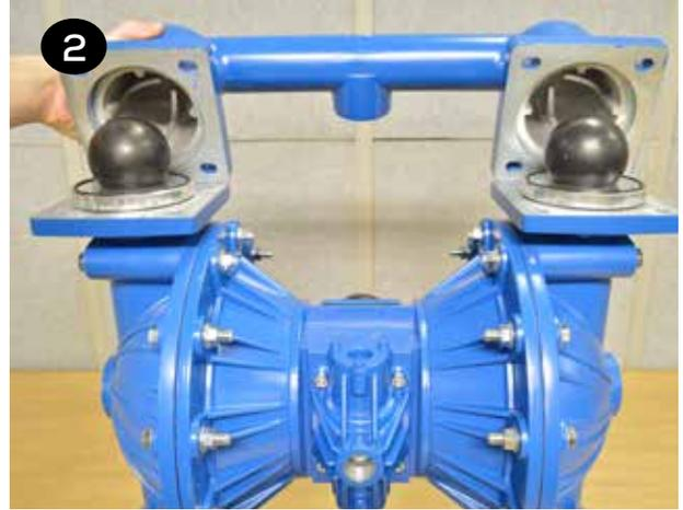
**3** Repeat the above steps for the suction manifold (item 12). The seat o-rings, valve seats and valve balls (items 13, 14, & 15) are located in the liquid chambers (item 18).
