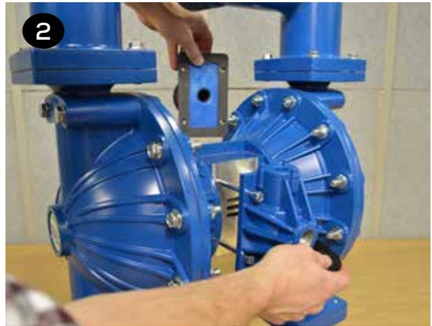
❸ Place the new gasket (item 38) on the air valve (item 3) and ensure the slots in the gasket align with the slots in the air valve and valve plate (item 10).
