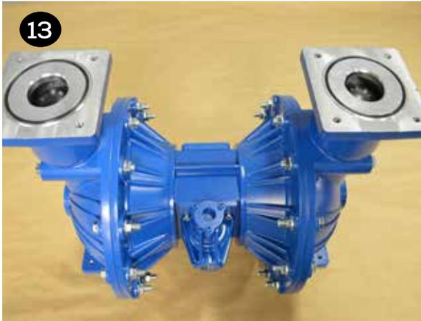
**14** Place the valve seats (item 14) into the seat bore in the liquid chamber (item 18). Place the suction manifold (item 12) atop the pump, install, tighten and torque the (8) manifold bolts (item 11).
