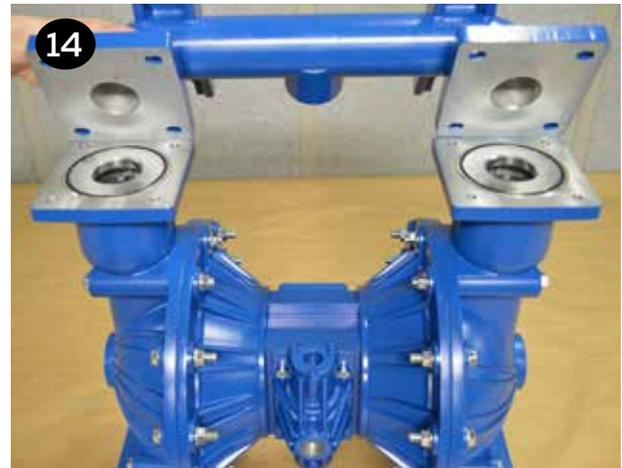
**15** Stand the pump upright onto the suction manifold feet. Place the valve seat o-rings (item 13) into both sides of the valve seat. Place the seat on the liquid chamber (item 18). Place the valve balls (item 15) on the seats and discharge manifold (item 39) atop the components that are stacked on top of the liquid chambers. Install, tighten and torque the (8) manifold bolts (item 11).
