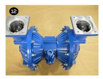
For pumps fitted with metal or PTFE valve seats (item 14), place the valve seat o-rings (item 13) into the glands on both sides of the valve seat. Pumps fitted with rubber or TPE seats do not require valve seat o-rings. All seats are symmetrical, i.e. there is no top or bottom.
