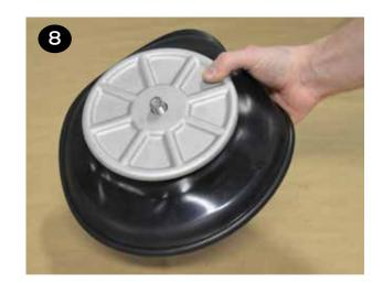
The other diaphragm(s) (items 21/22) and inner/outer plates (items 19 & 23) can be installed onto the opposite end of the shaft (item 32).
