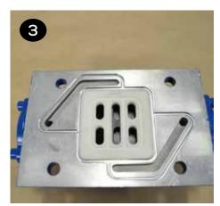
Insert the (4) cap screws & washers (items 1 & 2) through the valve body and gasket (items 3 & 36) and place onto the center section (item 35). Ensure the slide valve and valve plate (items 9 & 10) are in place and the valve sits flat on the center section.
