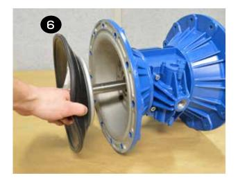
To remove the remaining diaphragm(s) (items 21/22) and plates (items 19 & 23) from the shaft (item 32), place the shaft in a vise. Using a 6-sided 30 mm wrench, remove the remaining diaphragm(s) and plates.
