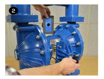
3 Place the new gasket (item 38) on the air valve (item 3) and ensure the slots in the gasket align with the slots in the air valve and valve plate (item 10).
