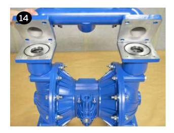
Stand the pump upright onto the suction manifold feet. Place the valve seat o-rings (item 13) into both sides of the valve seat. Place the seat on the liquid chamber (item 18). Place the valve balls (item 15) on the seats and discharge manifold (item 39) atop the components that are stacked on top of the liquid chambers. Install, tighten and torque the (8) manifold bolts (item 11).
