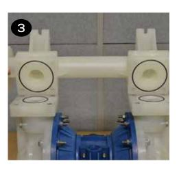
Remove both liquid chambers by removing the (12) bolts, washers & nuts (items 11, 12, 18 & 27) on each liquid chamber using a 17mm wrench and nuts can be removed using a 15mm wrench. Inspect and replace diaphragms if needed.
