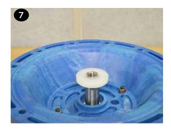
1 It may be easier to thread the molded in bolt into the shaft if the diaphragm(s) is inverted on one or both sides. This can be done by hand.
