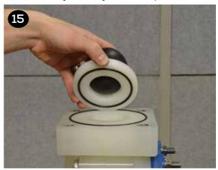
Place the valve balls (item 17) on the valve seats and discharge manifold (item 39) atop the components that are stacked on top of the liquid chambers. Install, tighten and torque the (8) manifold bots & washers (items 11 & 12).
