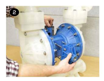
3 Place the new gasket (item 36) on the air valve (item 3) and ensure the slots in the gasket align with the slots in the air valve and valve plate (item 10).
