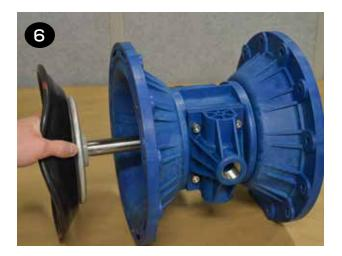
To remove the remaining diaphragm(s) (items 21/22) and plates (items 20 & 23) from the shaft (item 32), place the shaft in a vise. Using a 6-sided 30 mm wrench, remove the remaining diaphragm(s) and plates.
