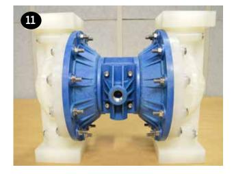
Flip the pump upside down and drop the suction valve balls (item 17) into the liquid chamber (item 19) ball cages.
