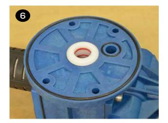
Install both air chambers (item 26) by placing one side on top of the center section (item 35). Ensure the air path hole of the center section lines up with the through hole in the air chamber. Insert the (4) bolts & washers (items 24 & 25) through the air chamber and center section.
