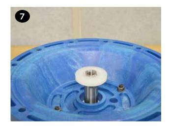
1 It may be easier to thread the molded in bolt into the shaft if the diaphragm(s) is inverted on one or both sides. This can be done by hand.
