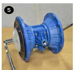
Remove the outer plate, diaphragm(s), and inner plate (items 20, 21/22 & 23) from the side that is loosened. Pull or push the shaft (item 32) and remaining plates and diaphragms out of the center section. If pulling, it may be easier to grip the diaphragm if it is inverted.
