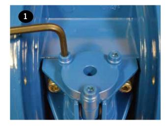
Plastic Air Valve - Remove and replace o-ring (item 5). Install cap (item 6) and tighten until groove for the retaining ring is visible. Install retaining ring (item 8).
