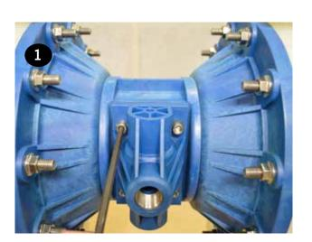
Pull the valve body and gasket (items 3 & 36) off the front of the center section (item 35) and the muffler plate gasket, muffler plate and muffler (items 37, 38 & 41) off the back.
