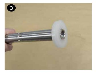
Apply a couple drops of a medium strength thread locker, such as Loctite® 246, to the molded in outer plate bolt (item 20). Thread the shaft (item 32) onto the molded in bolt until it is snug to the flat back side of the inner plate (item 22).
