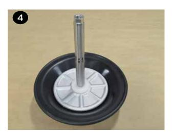
5 The shaft (item 32) and shaft o-rings (item 30) should retain the lubricant that was factory applied. If they appear dry, apply a light coat of lithium thickened grease. Avoid over lubrication as it can cause decreased performance of the air distribution system.
