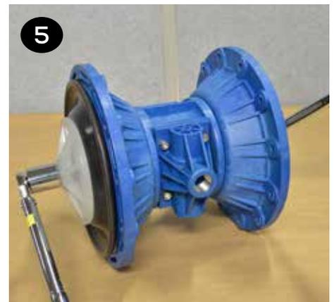
**6** Remove the outer plate, diaphragm(s), and inner plate (items 20, 21/22 & 23) from the side that is loosened. Pull or push the shaft (item 32) and remaining plates and diaphragms out of the center section. If pulling, it may be easier to grip the diaphragm if it is inverted.
