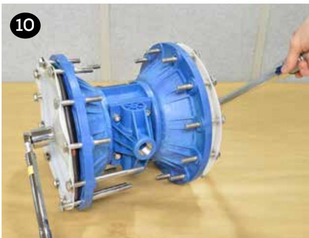
**11** Install the liquid chambers (item 19) by placing one side over the diaphragm. Start all bolts, washers & nuts (items 11, 12, 18 & 27) before tightening and torqueing. Torque all fasteners in a star pattern. Repeat to install the second liquid chamber. Ensure both chambers are orientated the same and that the inlet and outlet ports are vertical when facing the front of the pump as shown.
