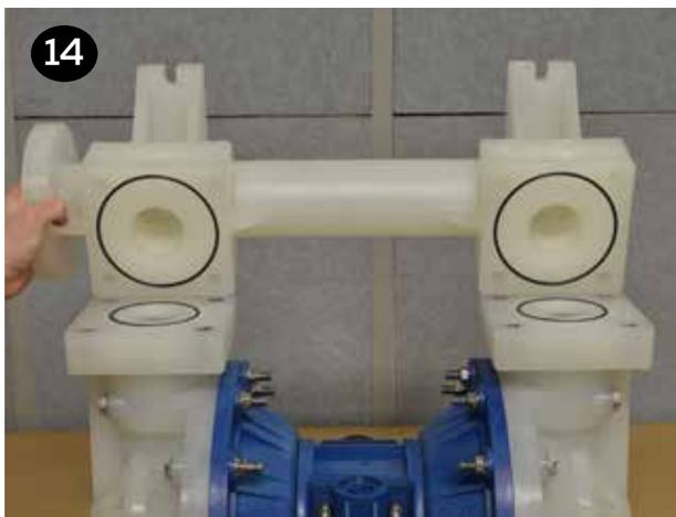
**15** Stand the pump upright onto the suction manifold feet (item 13). Place the large o-rings (item 15) into the glands in the face of the liquid chambers (item 19) followed by the small o-ring (item 14) in the gland of the valve seats (item 16). Place the valve seats on the liquid chambers with the o-ring down against the liquid chamber.
