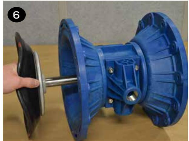
**7** To remove the remaining diaphragm(s) (items 21/22) and plates (items 20 & 23) from the shaft (item 32), place the shaft in a vise. Using a 6-sided 30 mm wrench, remove the remaining diaphragm(s) and plates.
