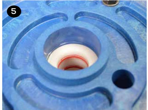
**6** Push the shaft (item 32) through the center of the shaft bushing (item 29). It is normal for this to be a tight fit, especially if the shaft and shaft o-rings (item 30) are in good condition.
