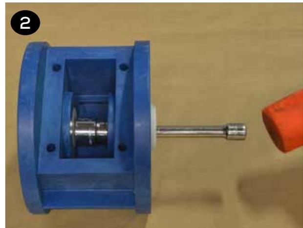
**3** Use the supplied grease packets to lightly grease the OD and ID o-rings (items 28 & 30) that come preinstalled in the new shaft bushings supplied in air end kits.
