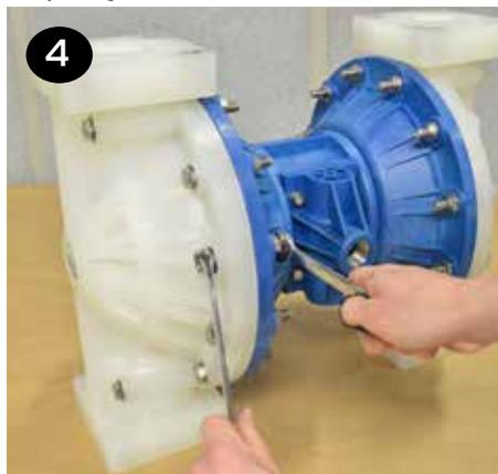
**5** To remove the diaphragms (items 21/22), begin by loosening the (2) outer plates (item 20) using two 30 mm wrenches. Use 6-sided sockets or wrenches to prevent damage to the hex portion of the outer plate.
