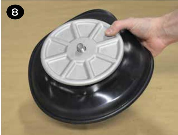
**9** The other diaphragm(s) (items 21/22) and inner/outer plates (items 20 & 23) can be installed onto the opposite end of the shaft (item 32).
