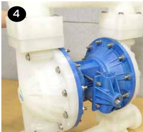
**5** Place the muffler gasket (item 37) over the (4) cap screws & lock washers (items 1 & 2) on the back side of the center section (item 35) followed by the muffler plate and muffler (items 38 & 41).
