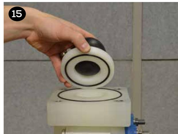
**16** Place the valve balls (item 17) on the valve seats and discharge manifold (item 39) atop the components that are stacked on top of the liquid chambers. Install, tighten and torque the (8) manifold bolts & washers (items 11 & 12).
