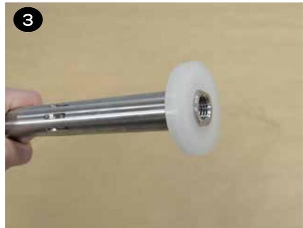
**4** Apply a couple drops of a medium strength thread locker, such as Loctite® 246, to the molded in outer plate bolt (item 20). Thread the shaft (item 32) onto the molded in bolt until it is snug to the flat back side of the inner plate (item 22).
