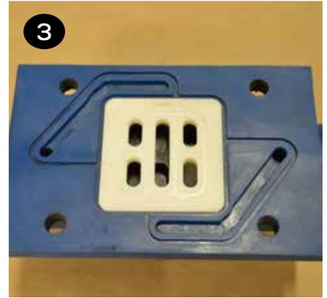
**4** Insert the (4) cap screws (item 1) through the valve body and gasket (items 3 & 36) and place onto the center section (item 35). Ensure the slide valve and valve plate (items 9 & 10) are in place and the valve sits flat on the center section.
