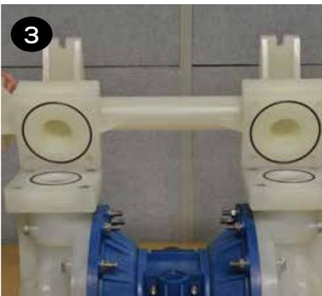
**4** Remove both liquid chambers by removing the (12) bolts, washers & nuts (items 11, 12, 18 & 27) on each liquid chamber using a 17mm wrench and nuts can be removed using a 15mm wrench. Inspect and replace diaphragms if needed.
