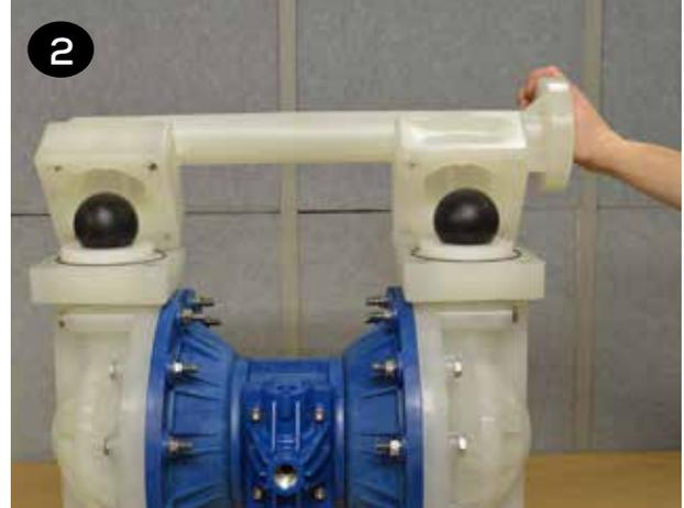
**3** Repeat the above steps for the suction manifold (item 13). The seat o-rings, valve seats and valve balls (items 14, 15, 16, & 17) are located in the liquid chambers (item 19).
