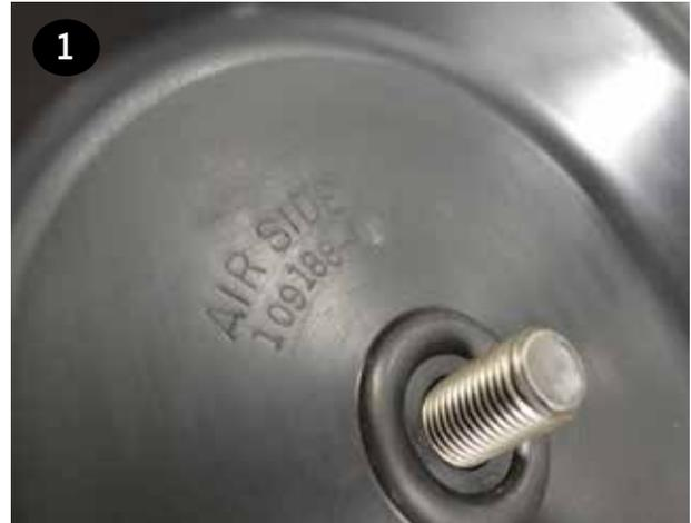
**2** Place the inner plate (item 23) over the molded-in bolt. Ensure the round recess in the plate faces the diaphragm (item 22).
