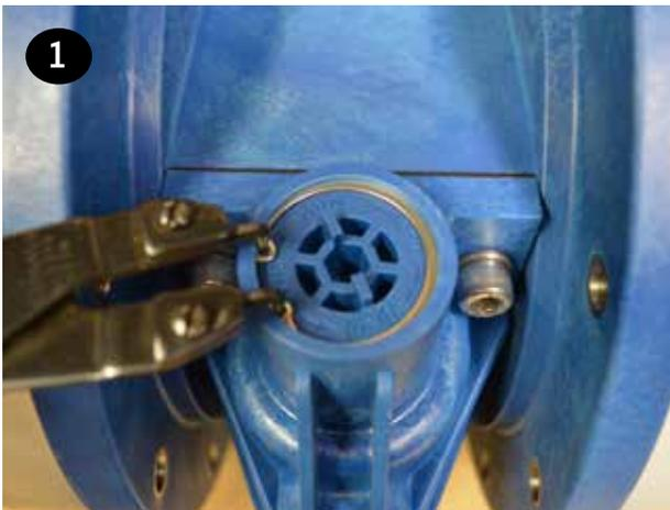
**1 Aluminum Air Valve** - To replace the valve cap o-rings (item 5), remove the (3) button head cap screws (item 7) using a 5mm hex wrench. Repeat for the remaining cap.
