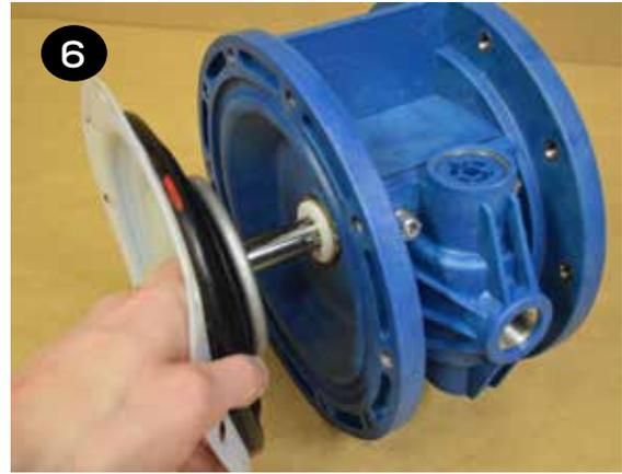
**7** To remove the remaining diaphragm(s) (items 20/21) and plates (items 19 & 22) from the shaft (item 27), place the shaft in a vise fitted with soft jaws. Using a 6-sided 30mm wrench, remove the remaining diaphragm(s) and plates. Soft jaws are required to prevent damaging the shaft. A damaged shaft will result in accelerated o-ring wear. Jaws can be fitted with wood, plastic, rubber, or other soft material to prevent shaft damage.
