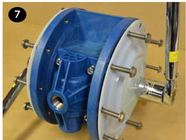
**Note:** When installing polytetrafluoroethylene (PTFE) diaphragms, it is important to tighten outer plates simultaneously (turning in opposite directions) to ensure tight fit.
