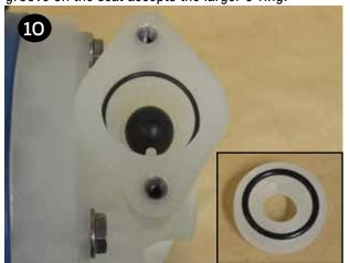
Check that the top of the seat (item 14) is about flush with the liquid chamber. Place the suction manifold (item 12) atop the pump. Tighten and torque the suction manifold bolts (item 11) in an "X" pattern.
