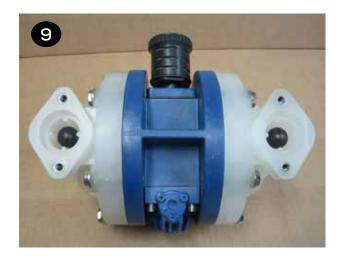
Place the larger valve seat o-rings (item 15) into the seat bores of the liquid chambers followed by the valve seats (item 14). Install the two smaller o-rings (item 13) into the face grooves in the valve seats. The seats are to be orientated so that the edge groove on the seat accepts the larger o-ring.
