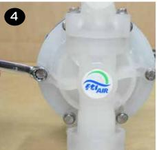
To remove the diaphragms (items 20/21), begin by loosening the (2) outer plates (item 19) using 2-20mm wrenches. Use 6-sided sockets or wrenches to prevent damage to the hex portion of the outer plate.
