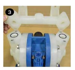
Remove both liquid chambers by removing the (6) bolts (items 17) on each liquid chamber using a 13mm (or ½") wrench. Inspect and replace diaphragms if needed.
