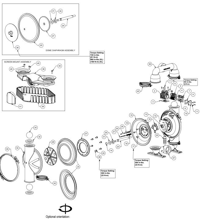
Optional orientation: To ease assembly of the TPE diaphragms, one of the diaphragms may be reversed. **Composite Repair Parts List - Elastomeric and TPE Fitted**
