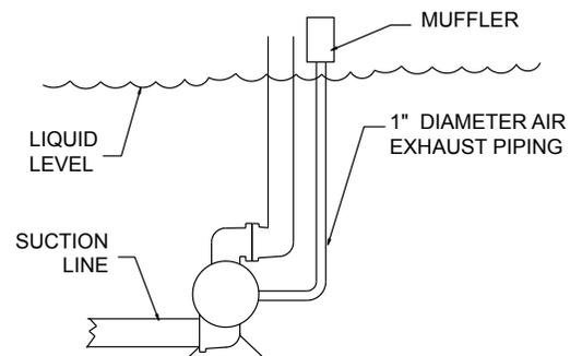
Pump can be submerged if the pump materials of construction are compatible with the liquid being pumped. The air exhaust must be piped above the liquid level. When the pumped product source is at a higher level than the pump (flooded suction condition), pipe the exhaust higher than the product source to prevent siphoning spills.
