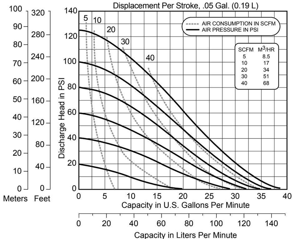
NOTE: Performance based on the following: PTFE fitted pump, flooded suction, water at ambient conditions. The use of other materials and varying hydraulic conditions may result in deviations in excess of 5%.
