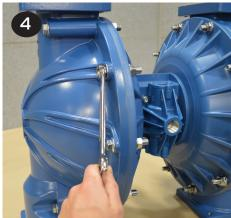
To remove the diaphragms (items 21/22), begin by loosening the (2) outer plates (item 20) using two 32 mm wrenches.
