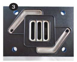
Insert the (4) cap screws & washers (items 1 & 2) through the valve body and gasket (items 3 & 37) and place onto the center section (item 36). Ensure the slide valve and valve plate (items 9 & 10) are in place and the valve sits flat on the center section.
