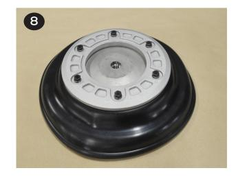
**9** The other diaphragm(s) (items 21/22) and inner/outer plates (items 20 & 23) can be installed onto the opposite end of the shaft (item 30).
