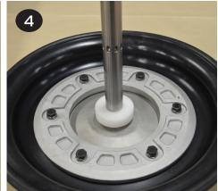
The shaft (item 33) and shaft o-rings (item 31) should retain the lubricant that was factory applied. If they appear dry, apply a light coat of lithium thickened grease. Avoid over-lubrication as it can cause decreased performance of the air distribution system.
