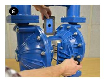
3 Place the new gasket (item 37) on the air valve (item 3) and ensure the slots in the gasket align with the slots in the air valve and valve plate (item 10).
