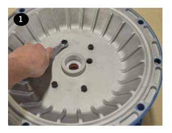
Remove and set aside the air valve (item 3) using a 6mm hex wrench (see Valve and Muffler Gasket Replacement section for more details). The shaft bushings can be removed by placing a large socket between the two bushings. Place and extension into the socket from one side of the center section (item 36). Tap with a rubber mallet to remove the bushing. Repeat for the remaining bushing.
