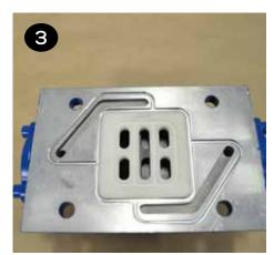
Insert the (4) cap screws & washers (items 1 & 2) through the valve body and gasket (items 3 & 37) and place onto the center section (item 36). Ensure the slide valve and valve plate (items 9 & 10) are in place and the valve sits flat on the center section.
