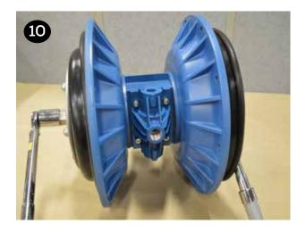
Install the liquid chambers (item 19) by placing one side over the diaphragm. Start all bolts & nuts (items 16, 18, 28) before tightening and torqueing. Torque all fasteners in a star pattern. Repeat to install the second liquid chamber. Ensure both chambers are orientated the same and that the inlet and outlet ports are vertical when facing the front of the pump as shown.
