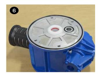
Install air chambers (item 27) by placing one side on top of the center section (item 36). Ensure the air path hole of the center section lines up with the through hole in the air chamber.
