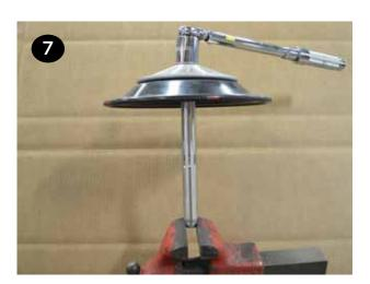
To remove diaphragms from inner & outer plates, remove the (6) bolts and washers (items 24, 25, & 26) that connect the inner plates to the outer plates using a 13 mm wrench.
