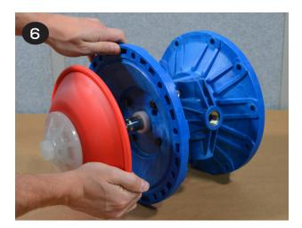
To remove the remaining diaphragm(s) (items 22/23) and plates (items 21 & 24) from the shaft (item 32), place the shaft in a vise fitted with soft jaws. Using a 6-sided 30mm wrench, remove the remaining diaphragm(s) and plates. Soft jaws are required to prevent damaging the shaft. A damaged shaft will result in accelerated o-ring wear. Jaws can be fitted with wood, plastic, rubber, or other soft material to prevent shaft damage.
