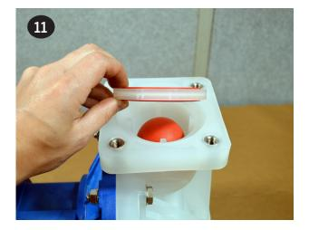
Place the suction manifold atop the pump and install, tighten and torque the (8) manifold bolts & washers (items 12 & 13).
