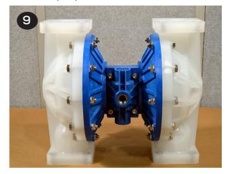
Flip the pump upside down and drop the suction valve balls (item 17) into the liquid chamber (item 20) ball cages.
