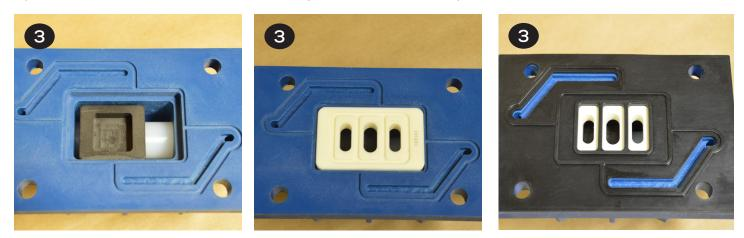
• Insert the (4) cap screws (item 1) through the valve body and gasket (items 3 & 6) and place onto the center section (item 35). Ensure the slide valve and valve plate (items 4 & 5) are in place and the valve sits flat on the center section.
