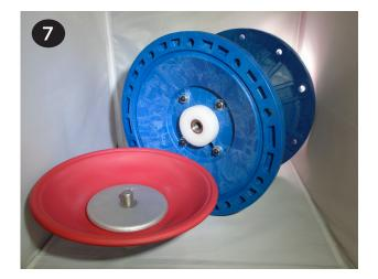
**8** Tighten and torque the outer plates (item 21) to 81.4 N-m (720 in-lbs).
