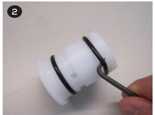
Aluminum Air Valve - To replace the valve cap o-rings (item 8), remove the (3) button head cap screws (item 11) using a 4 mm hex wrench. Repeat for the remaining cap.
