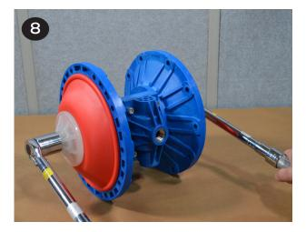
Install the liquid chambers (item 20) by placing one side over the diaphragm. Start all bolts, washers & nuts (items 18, 19, & 28) before tightening and torqueing. Torque all fasteners in a star pattern. Repeat to install the second liquid chamber. Ensure both chambers are orientated the same and that the inlet and outlet ports are vertical when facing the front of the pump as shown.
