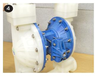
• Tighten and torque the (4) cap screws into the center section to 7.9 N-m (70 in-lbs).
