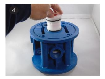
S Inspect the shaft (item 32) for damage. It is common for shafts to become grooved during service. Grooving is normally caused by carbonized oil and/or abrasive foreign material getting trapped between the seal and the shaft. Over time, deep grooves can form in the shaft. When that occurs, it is recommended that the shaft be replaced.
