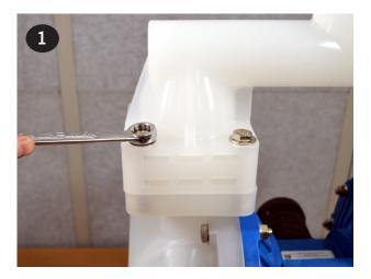
The discharge seat o-rings, valve seats, and valve balls (items 15, 16, & 17) can now be accessed and replaced if needed.
