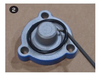
Remove the valve body (item 3) by removing the (4) socket head cap screws & lock washers (items 1 & 2) that attach the valve body to the center section (item 35) with a 6 mm hex wrench.
