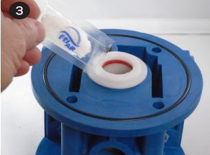
Remove and set aside the air valve (item 3) using a 6 mm hex wrench (see "Valve Replacement" section for more details). The shaft bushings (item 30) can be removed by placing a large socket between the two bushings. Place an extension into the socket from one side of the center section. Tap with a rubber mallet to remove the bushing. Repeat for the remaining bushing.
