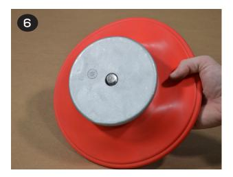
The other diaphragm(s) (items 22/23), inner/ outer plates (items 21 & 24) and bump stop (item 39) can be installed onto the opposite end of the shaft (item 32).
