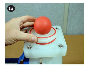
Place the valve balls (item 17) on the valve seats and discharge manifold (item 37) atop the components that are stacked on top of the liquid chambers. Install, tighten and torque the (8) manifold bolts & washers (items 12 & 13).
