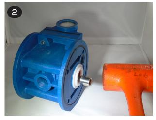
• Insert both bushings into the center section. Ensure the bushing is fully installed.
