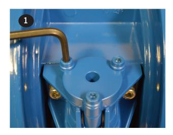
Aluminum Air Valve - Remove and replace o-ring (item 8). Install cap (item 9), tighten, and torque the valve cap screws (item 11) to 6.8 N-m (60 in-lbs). Repeat for the remaining cap.
