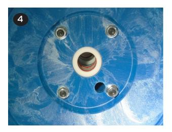
• Push the shaft (item 32) through the bump stop (item 39) and center of the shaft bushing (item 30). It is normal for this to be a tight fit, especially if the shaft and shaft o-rings (item 31) are in good condition.
