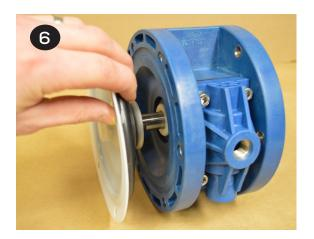
To remove the remaining diaphragm(s) (items 20/21) and plates (items 19 & 22) from the shaft (item 27), place the shaft in a vise fitted with soft jaws. Using a 6-sided 20mm wrench, remove the remaining diaphragm(s) and plates. Soft jaws are required to prevent damaging the shaft. A damaged shaft will result in accelerated o-ring wear. Jaws can be fitted with wood, plastic, rubber, or other soft material to prevent shaft damage.
