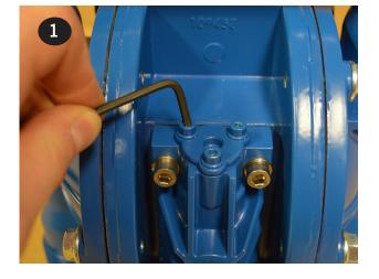
Plastic Air Valve - Remove and replace o-ring (item 5). Insert cap (item 6) and push down until groove for the retaining ring is visible. Make sure to lubricate the o-rings prior to inserting into the valve body with a compatible lubricant.
