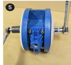
Remove the outer plate, diaphragm(s), and inner plate (items 19, 20/21 & 22) from the side that is loosened. Pull or push the shaft (item 27) and remaining plates and diaphragms out of the center section. If pulling, it may be easier to grip the diaphragm if it is inverted.
