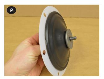
Apply a couple drops of a medium strength thread locker, such as Loctite® 246, to the molded in outer plate bolt (item 19). Thread the shaft (item 27) onto the molded in bolt until it is snug to the flat back side of the inner plate (item 22).
